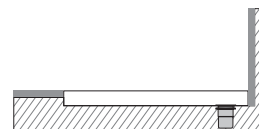
Can be embedded into the floor or glued onto the surface
